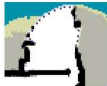
Figure 3: Occupancy Map Used for Exploration “Obstacle” cells are black, “clear” cells are white, “unknown” cells are grey. Frontier cells are marked by small circles.
